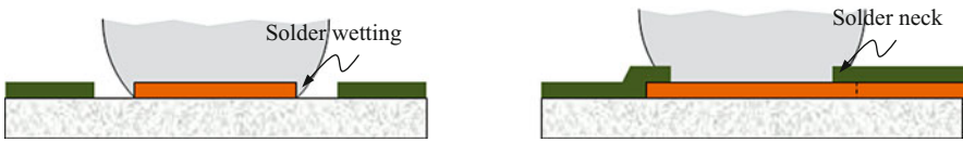
Fig. 9.3 Wetting of solder on sidewalls of NSMD pad and solder necking on SMD pad
