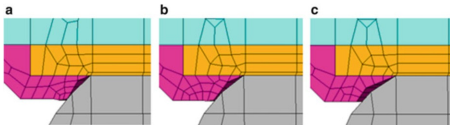
Fig. 10.41 Finite element model of the three different polyimide layouts: (a) PI layout 1, (b) PI layout 2, and (c) PI layout 3
