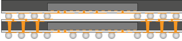
Fig. 4.13 A conceptual PoP based on fan-out WLCSP. Through-mold via (TMV) is drilled through bottom fan-out package to make the front (active side) to back vertical interconnections. Backside rerouting is needed for connecting the top chip. In case of full area array, fan-in routing could be made on the back side of bottom package
