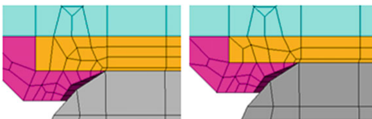
Fig. 10.42 Finite element models of two different copper UBM thicknesses
