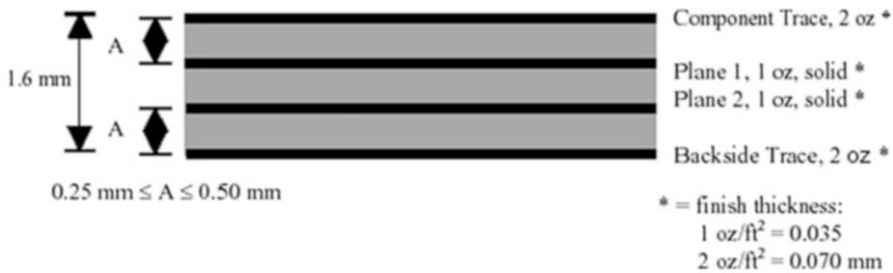
Fig. 7.8 Cross section of multilayer PCB in JEDEC standard
